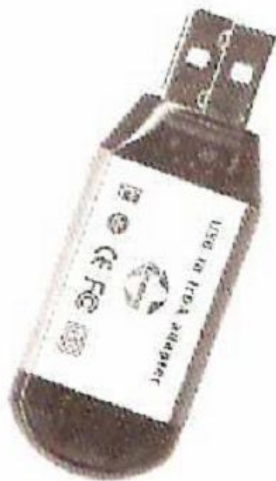
Rys. 8.5. Karta interfejsu (adapter) IrDA
